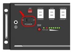
4) The one with **empty Link Port 0** is the **Master Battery** Module, others are slaves (1 master battery configure with maximum 15 slave batteries):
